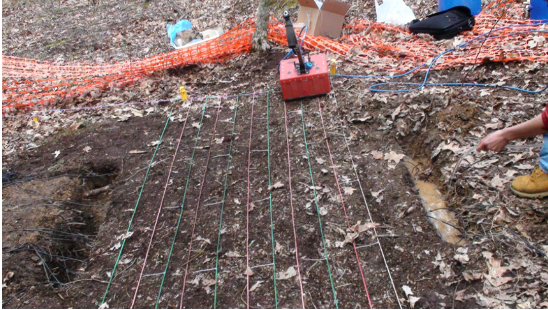
Experimental setup of time-lapsed GPR scanning and real-time soil moisture monitoring with introduced water infiltration in a hillslope at the Shale Hills Catchment.
